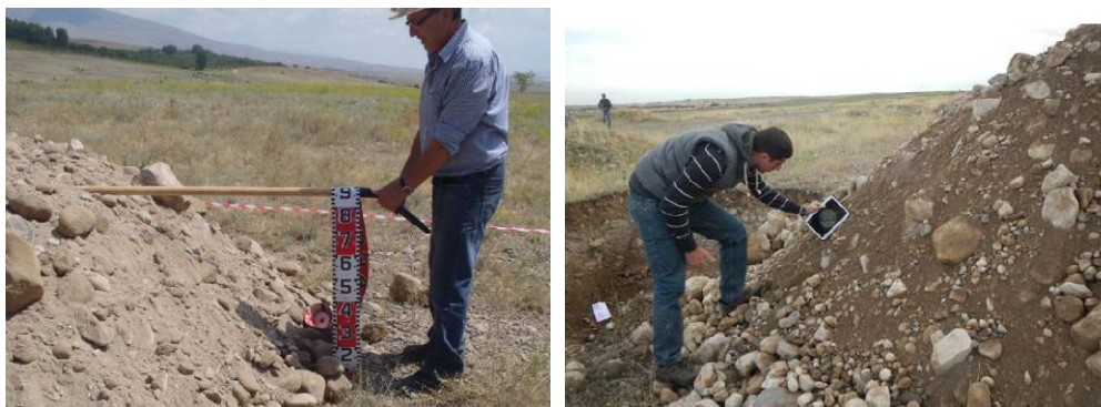
Figure 4-3-7.7 Circumstances in the Repose Angle Measurement
