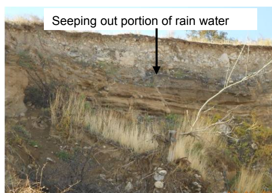
Figure 4-3-6.6 Conditions Observed on the Cliff Slope of Sand-and-Gravels
