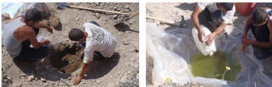
Figure 4-3-7.5 Circumstances in the Field Density Test
