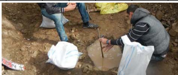
Figure 4-3-7.6 Circumstances in the Field Permeability Test
